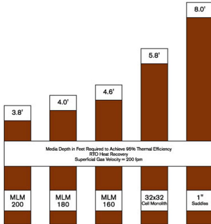
**Figure 5. Depth of heat recovery media needed to achieve 95 percent thermal efficiency.**
