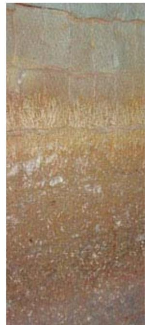
**Figure 4. Distinct settlement lines and impressions into insulation along inside of the canister walls caused by collapse of the saddle**
