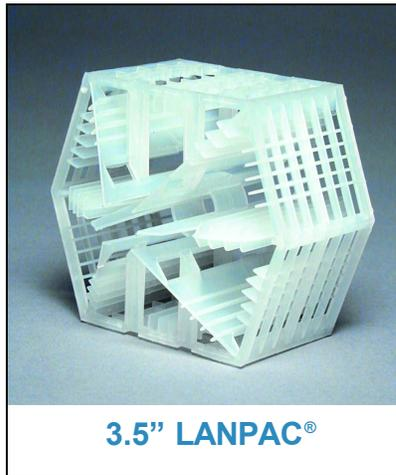
The efficiency of tower packings is expressed as the height of transfer unit (HTU), which is the depth of packing needed to accomplish a given degree of purification. The smaller the HTU of a given packing, the more efficient that packing is, so the smaller an air stripper will need to be to do the job.
