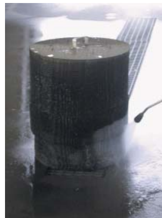
The cleaning of the HD Q-PAC® is shown (left) as well the result (right).
