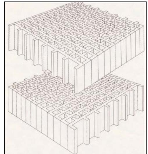
Figure 2. MLM® structured RTO heat recovery media from Lantec Products. Note that by rotating the plates of successive layers 90° that each successive layer is supported by the lower layer of media.
