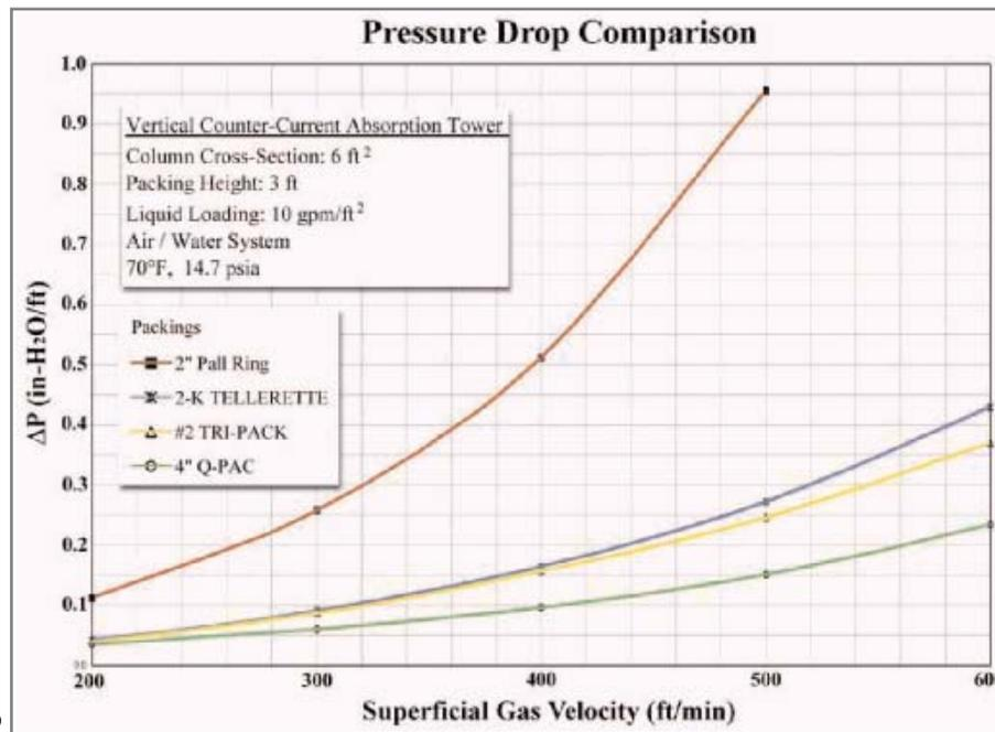
Figure 3. Pressure drop of Q-PAC compared to several competitive packing products.
