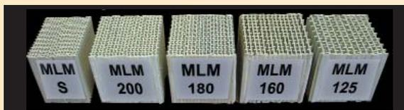
**MLM's parallel-plate structure** packs more ceramic material into each cubic foot (over 3 times more surface area than saddles) with less resistance to air flow. The result is a unique combination of high heat capacity, rapid heat transfer, low pressure drop, and great resistance to plugging by particulates. When MLM-S is used as the design basis rather than 1" saddles, heat recovery beds can be ~50% shorter.
